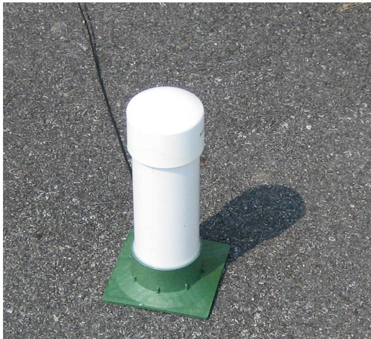
**Figure 3: Picture of Quadrafilar helix antenna**
